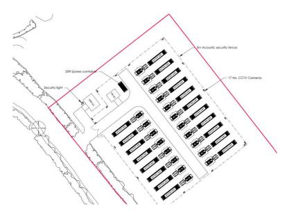
6.2 In addition, an underground cable will run from the battery storage units to the Upton Heath substation. The cable runs a distance of approximately 1km to the electrical substation, which will cross the A350 Blandford Road North. Access to the main site will be via the south west of the site, onto the existing road which serves a nearby telecommunications site.
